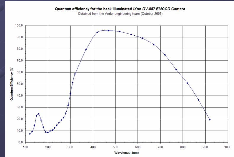
Thinned, Back-illuminated, ARC, -87C water cooling, 512 x 512 (16  $\mu$ m) pixels, 8.2 x 8.2<sup>19</sup>mm
