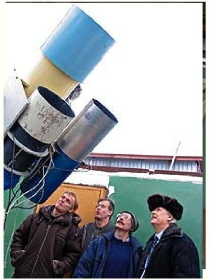
The main telescope is Richter-Slefogt, D=355 mm, D/F=2.3 CCD is Apogee Alta U16 that give us 6 sq.deg.
